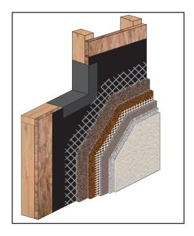
Parex Armourwall 100 Stucco is a 1-coat system providing a durable exterior stucco façade with unique, refined aesthetic appeal. This minimum 3/8" thick system can be installed at greater thicknesses in accordance with ASTM C926 as required for fire resistance rated assemblies or STC ratings. Enhanced Krak-Shield crack-resistance is available for all configurations by incorporating a reinforced leveling coat prior to application of the finish.
