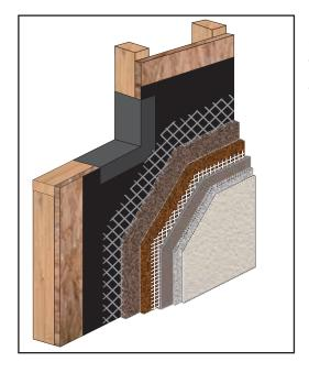
Parex Armourwall 300 Stucco is a 3-coat system that provides a durable exterior stucco façade with unique, refined aesthetic appeal. This 3/4" thick system can be installed at greater thicknesses in accordance with ASTM C926 as required for fire resistance rated assemblies or STC ratings. Enhanced Krak-Shield crack resistance is available for all configurations by incorporating a reinforced leveling coat prior to application of the finish.
